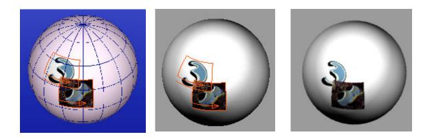
The bounding texture usage has been improved to allow bounding surface transformations both in Render mode and ExTrace images similarly. For example, rotating bounding surface updates the corresponding bounding texture in Render mode as seen in the two images below.
