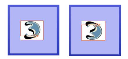
With cylindrical surfaces the defined texture area may go over the seam of the surface and the result will thus go around the object. This can be easily fixed with wrapping and rotation commands remembering that the Texture Marker arrow on the surface always gives the direction of the Texture Image horizontal axis.
