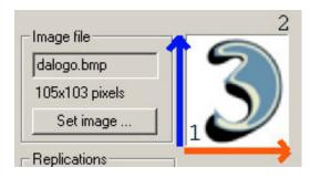
Below we can see the same texture positioned on a plane primitive. The points 1 and 2 indicate the order and position of the two corners given with the mouse. The blue and red axis give the vertical and horizontal axis on the surface. The Texture Marker arrow (thin red line on and around the image) shows the direction of the Texture Image horizontal axis on the surface *at all times*.
