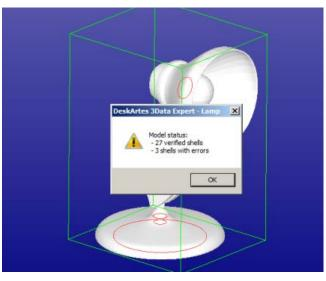
The message indicates that there are 27 verified shells, of which three shells contain errors. The display also shows red *Gap curves* through the surfaces. Gaps are an error type you must fix during the repair process. Note that the model is now displayed completely in white. This color indicates that the normals are already oriented consistently and correctly outwards.
