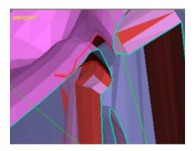
We can see that both the disjoint shells are more or less at the same distance from each other along the open edge. The approximate distance can be measured using the *Dimensions > Distance* command and it will give approximately 0.05 units (you can also use the icon to start the *Distance* command).
