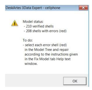
This indicates that most shells have errors and we should use Model Tree and Help Text to repair the model.
