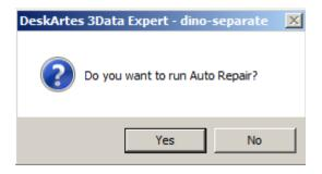
The Auto Repair process is not well suited for fixing models with the errors we have now. In the Auto Repair process each shell is repaired individually into a solid shell. In this case connecting the separate shells at the open edges would yield the correct result. We will
