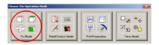
The normal way to begin repairing a model is to start with the Fix Model mode. To start fixing
