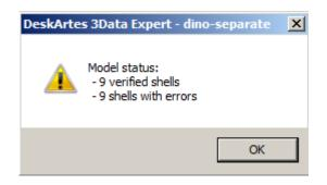
This is the result of the automatic analysis (a separate verification of the input model with *Fix Model* > *Verify Shells* would yield similar result). We can see that the 9 shells in the Model Tree are all separated by thin gaps.
